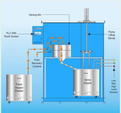
Powder kitchen is the system which organizes your coating process & keeps the coating zone free of powder spillage. All powder being used is contained in the kitchen.
